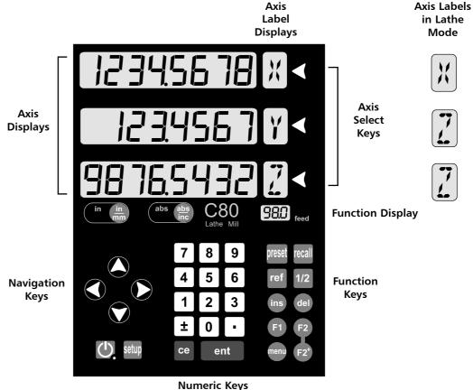
For more information about the use of the Navigation Keys and the Function Keys, see the sections on Setup and Special Functions, later in this guide.
