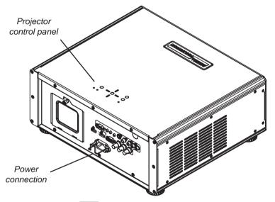
Press POWER ON on the remote control or POWER (1) on the projector control panel to switch the projector ON. The power indicator on the control panel will flash blue for approximately 30 seconds, whilst the lamp comes up to full brightness. When the projector is ready for use, the power indicator will show a steady blue.
